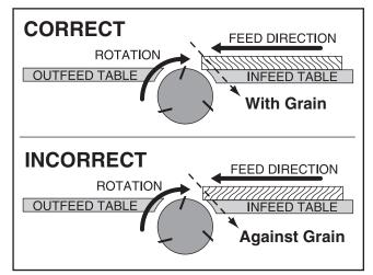
Figure 26. Correct and incorrect grain alignment with cutterhead.
